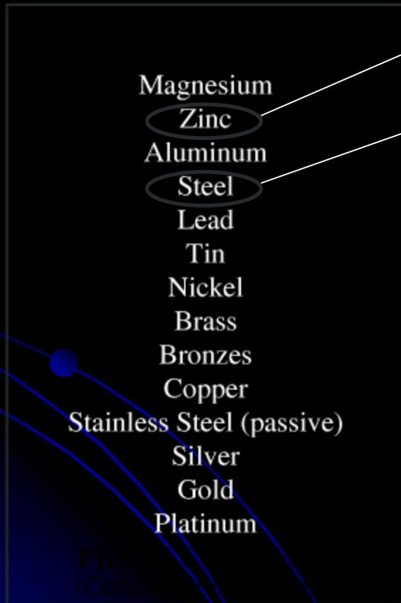
**This arrangement of metals determines what metal will be the anode and cathode when the two are put in a electrolytic cell (arrangement dependent on salt water as electrolyte).**
